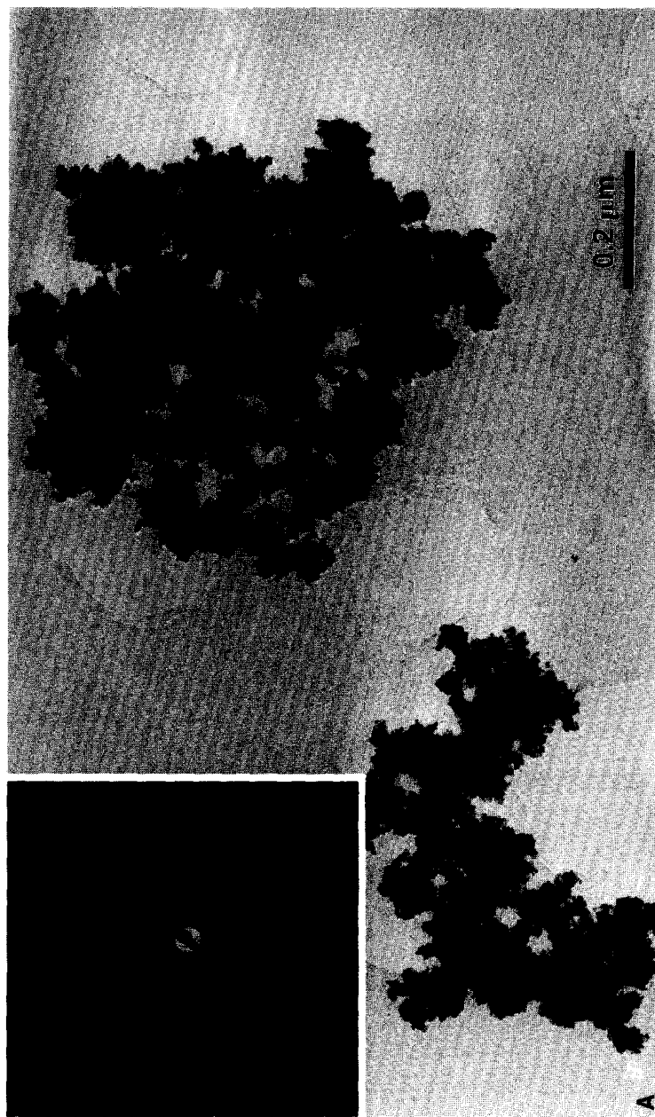
FIG. 1. Transmission electron micrographs of Pt-black. (A) Aggregates of finely divided fresh Pt-black. Inset: selected area electron diffraction (SAED) pattern. (B) An aggregate of Pt-473 with increased particle size. Inset: SAED pattern. (C) Rounded sintered Pt-633 particles, opaque to electrons.
